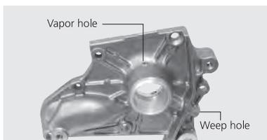
Quality materials are used to withstand heat, vibration and corrosion. Water channel is designed with optimal flow of coolant. Positioning of vapor hole and weep hole are key to prevent excess coolant from bearing and shaft contamination.
